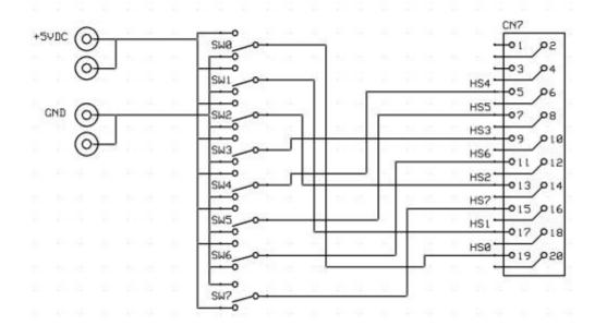
Use single pole double throw toggle switches for SW0...SW6. Use a single pole double throw momentary contact switch for SW7. Set the desired sound number (see the <u>Farfalla</u> sound map for examples) on SW0...SW6, then press the momentary SW7 to toggle the IRQ line. The corresponding sound or speech call should be played.
