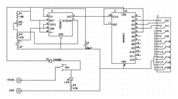
Rather than having individual toggle switches, this one just continuously cycles through the three address pins and ties all of the chip select pins Low so as to continuously toggle all output pins of the Driver board for easy testing with a logic probe.
