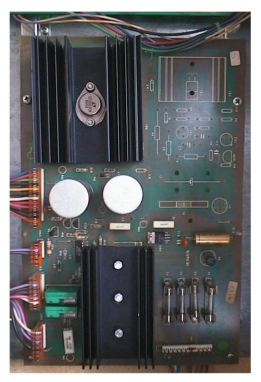
On their last regular game, Zaccaria introduced LED-based score displays, and a modified 1B1167 power supply board that eliminated the parts for the 170V high voltage displays. There is a jumper added to the back side of the board between CN5 pin 12 and TP1 to provide +12VDC to power the LEDs on the displays. Other than the missing parts, the board appears to be identical to the 1B1167/0.
