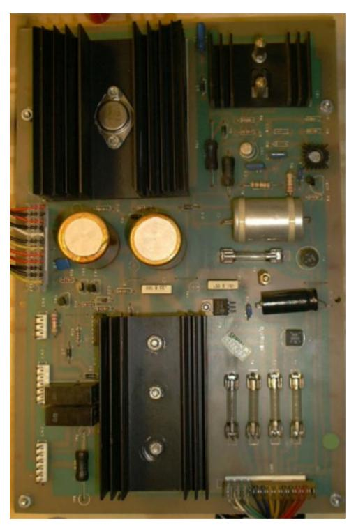
The power supply board takes the input voltage from the transformer in the main cabinet, and generates the +5, +12, +39, +170 and -5 voltages needed for the logic, lamps, solenoids, and display circuits.
