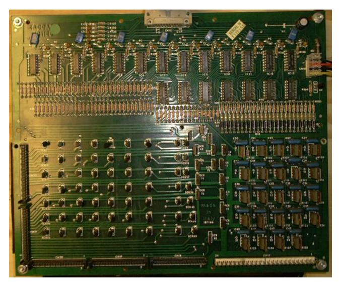
The driver board houses the lamp drive SCRs and the solenoid drive transistors. It takes a data signal from the CPU board via a short ribbon cable, and has Molex connectors for the controlled lamps and solenoids.
