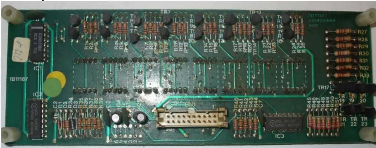
Picture by Laszlo The 1B11187 eight digit LED display.
